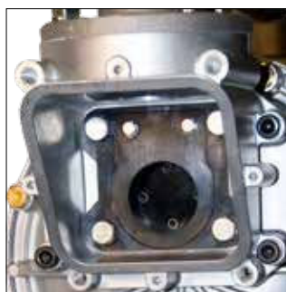
Only 4 bolts to access flap valves
