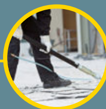
Compressed air lances
