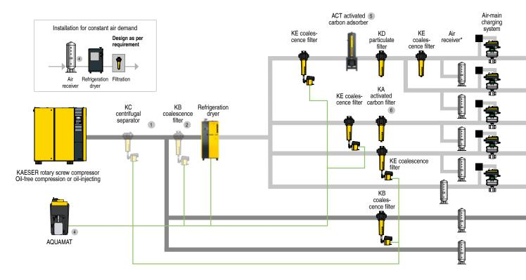
Compressed air treatment with a refrigeration dryer (pressure dew point to +3 °C)
