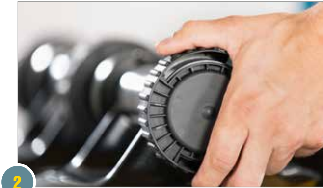
2 The clamping nuts on the cartridge screw connection are then loosened.
