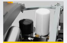
Oil separation with spin-on cartridges
