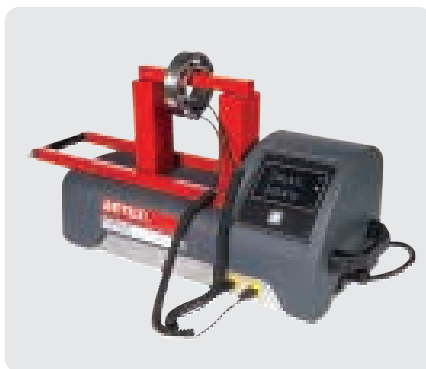
Heating a hanging workpiece, for small bores
