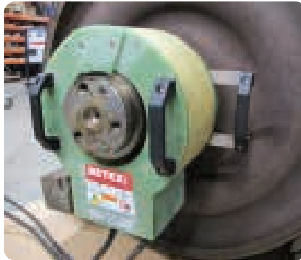
Heating bearing rings for dismounting
